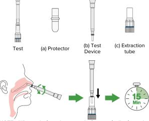
NOTE: When placing the test device vertically into the extraction tube, the edge of the extraction tube must reach the top of the supporting ring. If not, this may lead to lateral flow failure, resulting in an incorrect result or invalid result.
