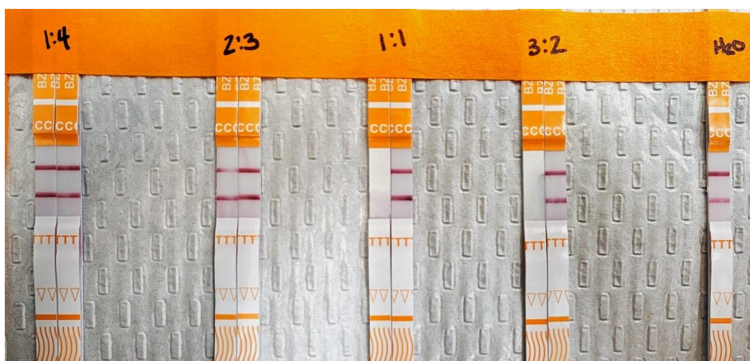
Figure 2. Effect of increasing amount of organic solvent on test strip results. The ratio of organic solvent:water increases from left to right, with results from pure water on the right hand side for reference. For each ratio, the acetonitrile:water mixture is on the left and the methanol:water mixture is on the right. Note the lack of development of the control band (top band) and the test band (lower band) at high (1:1 and 3:2) acetonitrile:water ratios. No analyte was added to solution so that the test band would also be developed.
